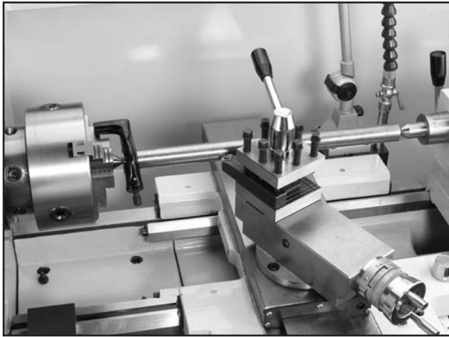
Figure 37. Example of stock mounted between the centers.
